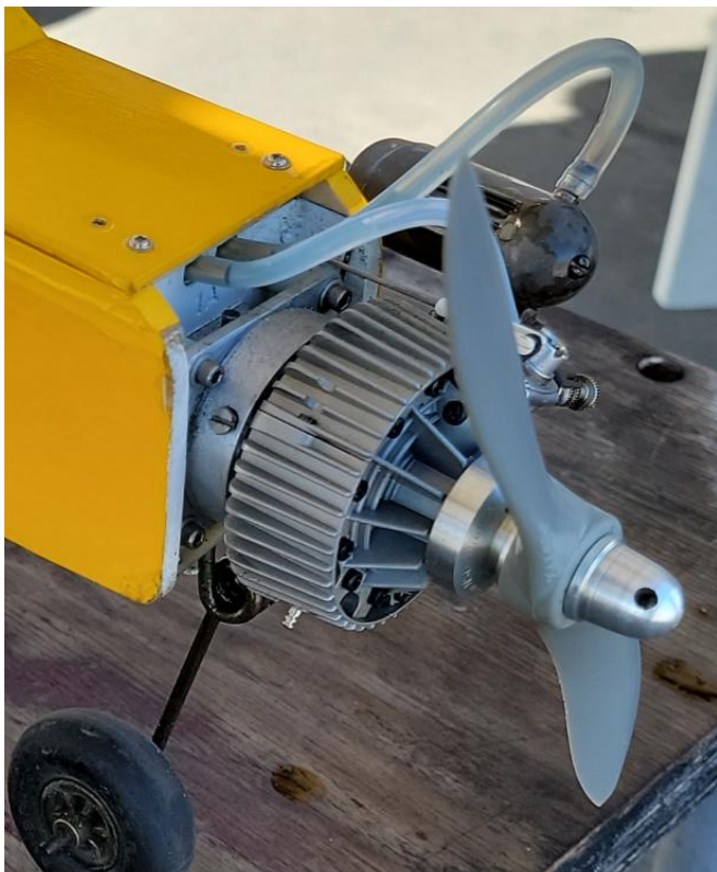
A close-up of the Wankel rotary engine
